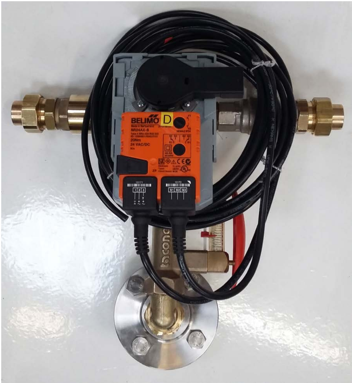
BAF pump outlet assembly
