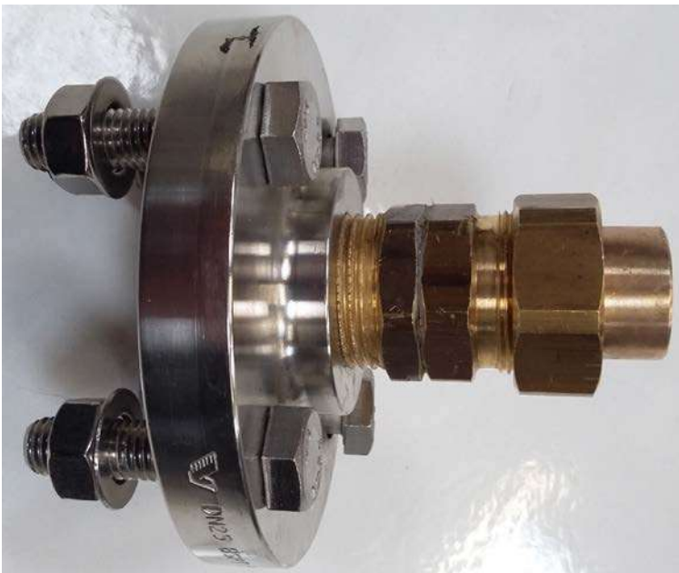
BAF pump inlet assembly
