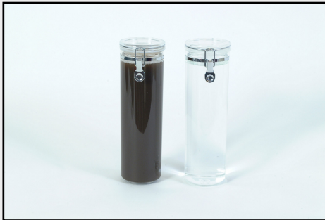
Hilton Olympia heating system water samples: Visual appearance and laboratory analysis, 2003-2004.
